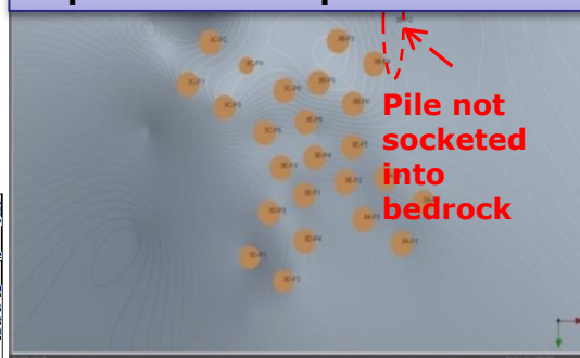
Visualization of problematic pile socket
