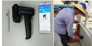
Reading RFID tag after concreting
